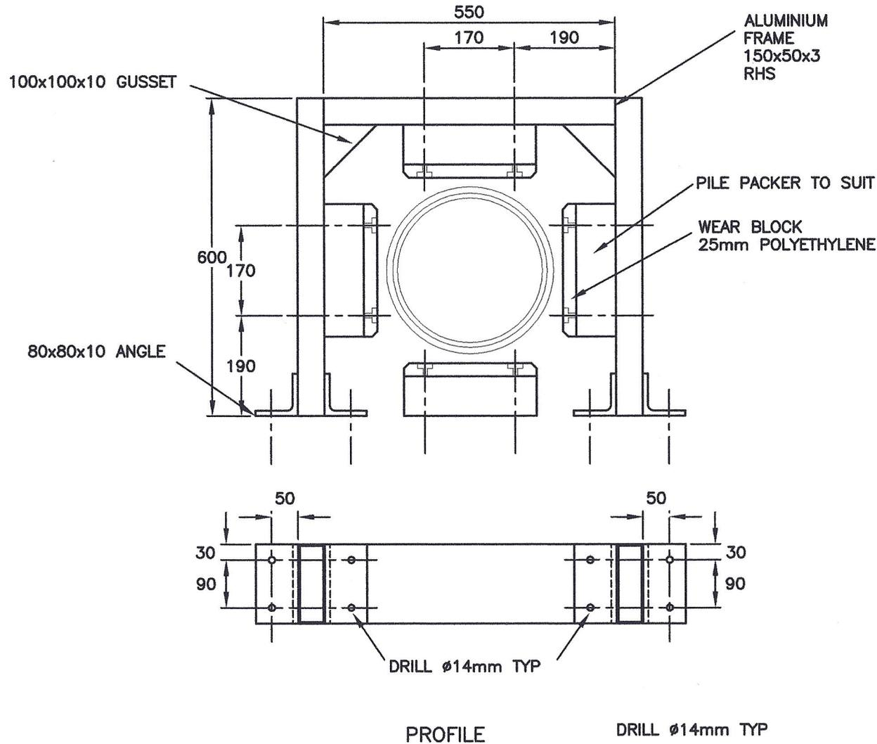
NOTE—ALL STRUCTURE IS FULLY WELDED WITH A FILLET OF 5mm
