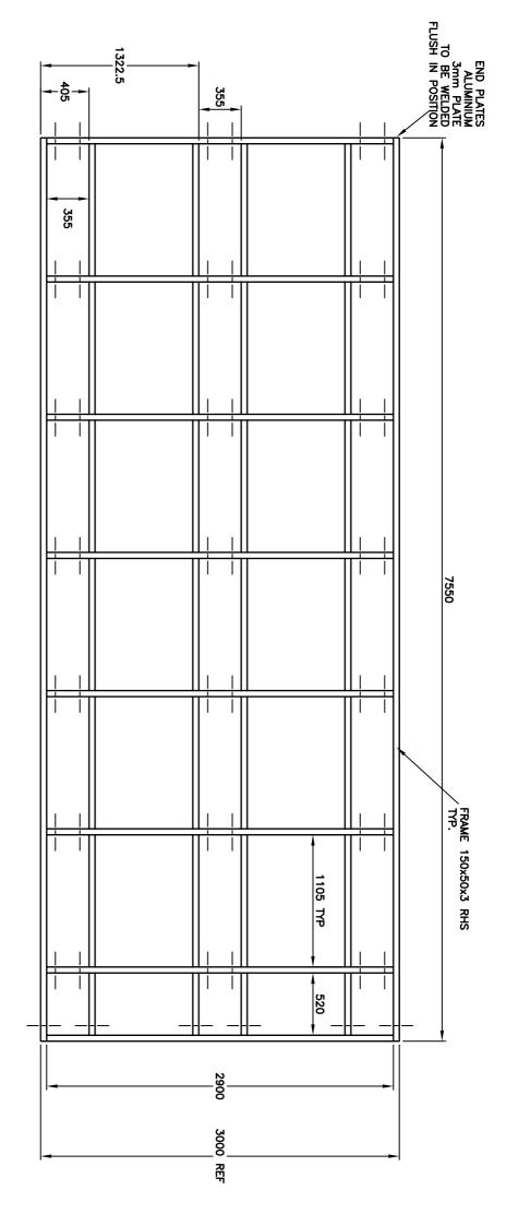
NOTE- STRUCTURE IS TO BE FULLY WELDED. HOLES ARE TO BE DRILLED IN UNDERSIDE OF MEMBERS TO ALLOW FOR WATER AND MOISTURE TO ESCAPE.
