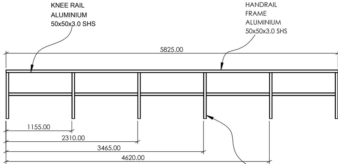
NOTE: ENSURE VERTICAL POSTS LINE UP WITH JOISTS ON MAIN FRAME SEE DWG 7142 FOR DETAIL
