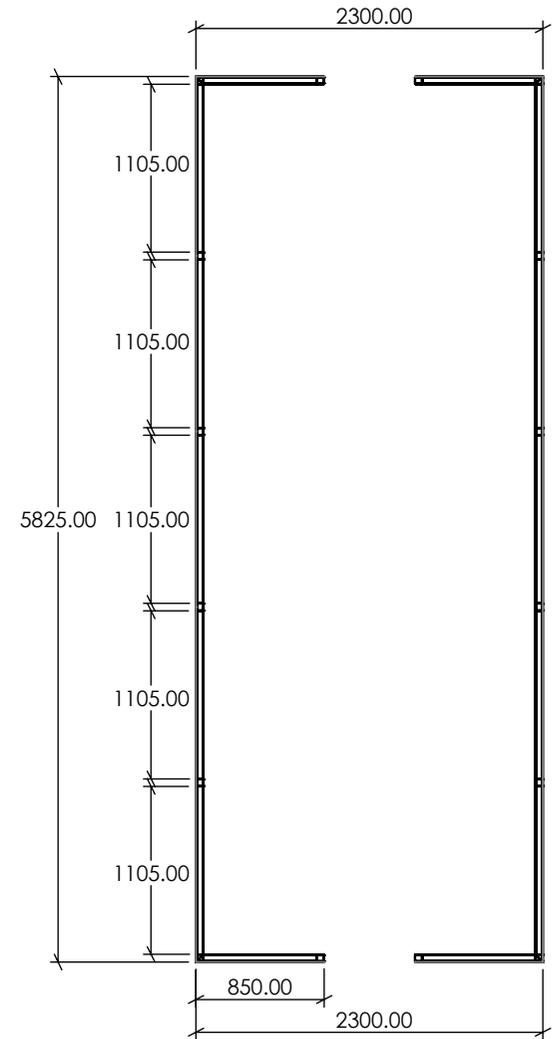
NOTE -ALL STRUCTURE IS FULLY WELDED WITH A NOMINAL FILLET RADIUS OF 5mm.
