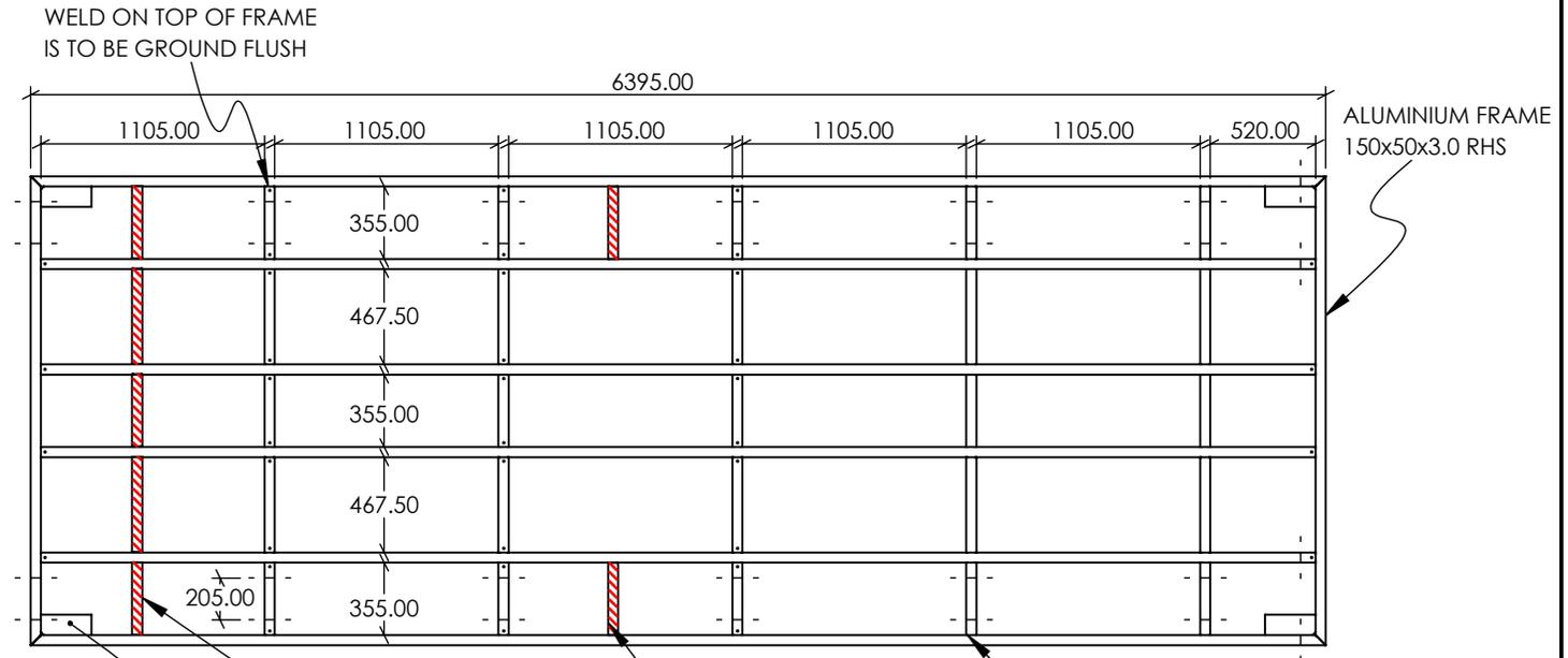
ALUMINIUM 100x10 FLATBAR x250mm WELDED FLUSH WITH FRAME. CHAMFER CORNER TO CLEAR WELD.
