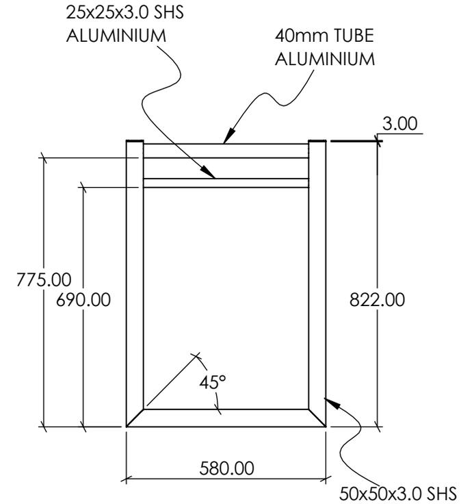
NOTE -STRUCTURE IS TO BE FULLY WELDED. HOLES ARE TO BE DRILLED ON UNDERSIDE OF MEMBERS TO ALLOW FOR WATER AND MOISTURE TO ESCAPE.
