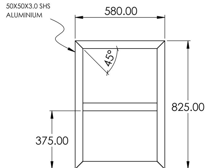
NOTE -STRUCTURE IS TO BE FULLY WELDED. HOLES ARE TO BE DRILLED IN UNDERSIDE OF MEMBERS TO ALLOW FOR WATER AND MOISTURE TO ESCAPE.
