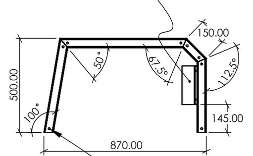
DRAINAGE HOLES TO BE DRILLED IN UNDERSIDE OF FRAME. Ø 5mm, 20mm FROM THE END OF EACH SEALED MEMBER. AS SHOWN.
