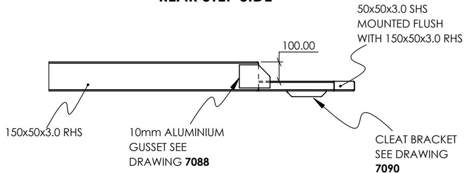
**NOTE** -STRUCTURE IS TO BE FULLY WELDED. HOLES ARE TO BE DRILLED IN UNDERSIDE OF MEMBERS TO ALLOW FOR WATER AND MOISTURE TO ESCAPE.
