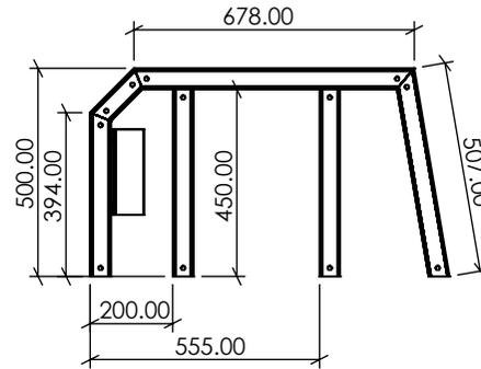
MOUNT CLEAT BRACKET (80x80x10 EA) 20mm FROM JOIN TO CLEAR WELD REFER TO DWG NO. 7087
